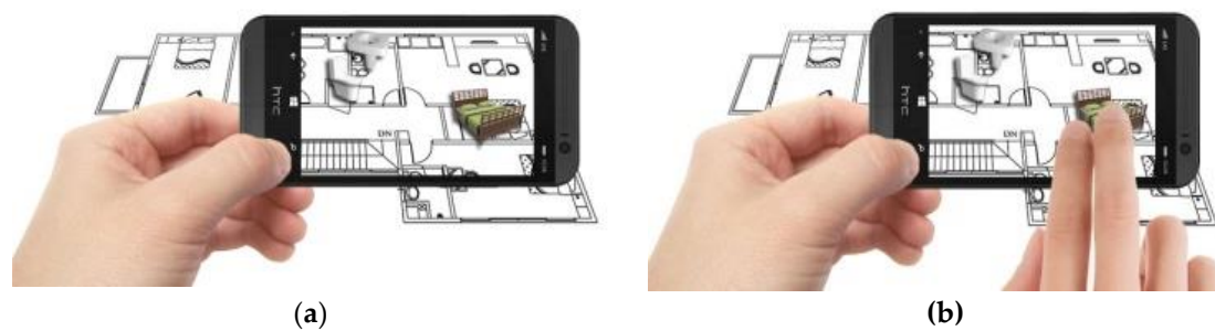
Figure 3. (a) AR-based simulation of 2D interior design layout plans and integration of 3D images of interior design symbols; (b) Students can evaluate different design decisions by moving 3D objects in AR on their mobile phone screens.
